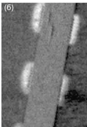
(a) – sample structure, (b) – capacitance contrast dC/dV , (B) – topography ( measured separately ) Scan size 3.5x5 \mu\text{m}
