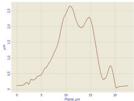
Fig.1. Living polymorphonuclear neutrophils and profile of living cells in liquid obtained in semicontact mode with contact Si probes CSG 11. Scan rate about 2 line/sec.
